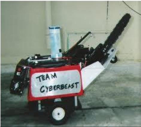
Gladiator Rodney: Yes, that's an electric chainsaw on an autonomous robot (be afraid). Note the 38KHz Infrared Pringles can beacon on top (homebrewed) and 1000 Watt inverter on back.
