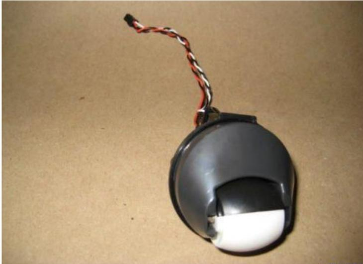
The heart and mind of the "Rodney Jr" system is the Roomba mobility sensor... all the robot wants to know is whether it is moving or not. He eventually learns the motion patterns which provide the most magnitude or displacement.
